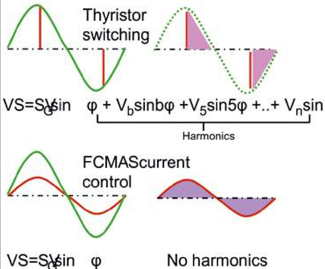
FCMA Soft Starters control the amplitude of Motor current without distorting the current waveform. This leads to zero harmonics and substantially low starting current.
